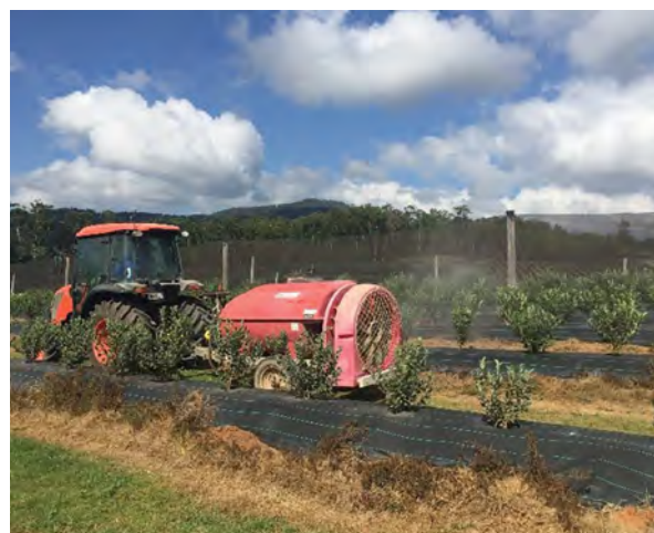
Figure 173. An axial air-blast sprayer.
