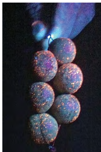
Figure 185. Using fluorescent dyes to demonstrate coverage.
