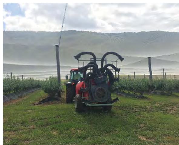
Figure 171. A ducted air sprayer.
