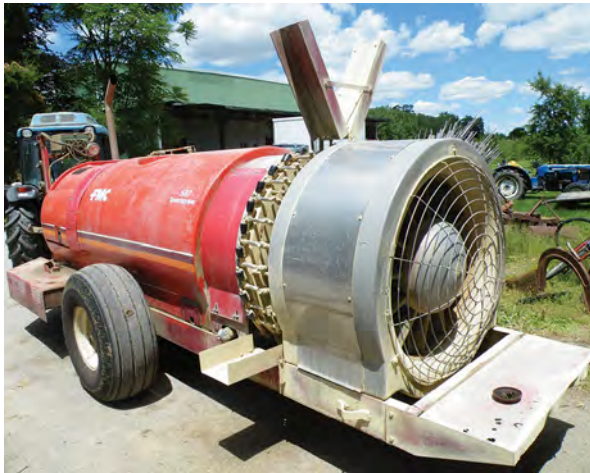
Figure 177. Deflectors on an air-blast sprayer. Photo: Deveau (2015).
