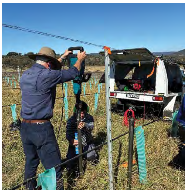
Figure 26. Soil cores being taken to map root distribution and calculate water holding capacity. Photos: Dr Jason Smith, Charles Sturt University.
