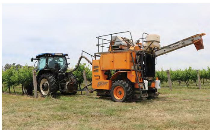
Figure 18. A Pellenc pull-behind harvester is used to shake the Pinot Gris vines.
