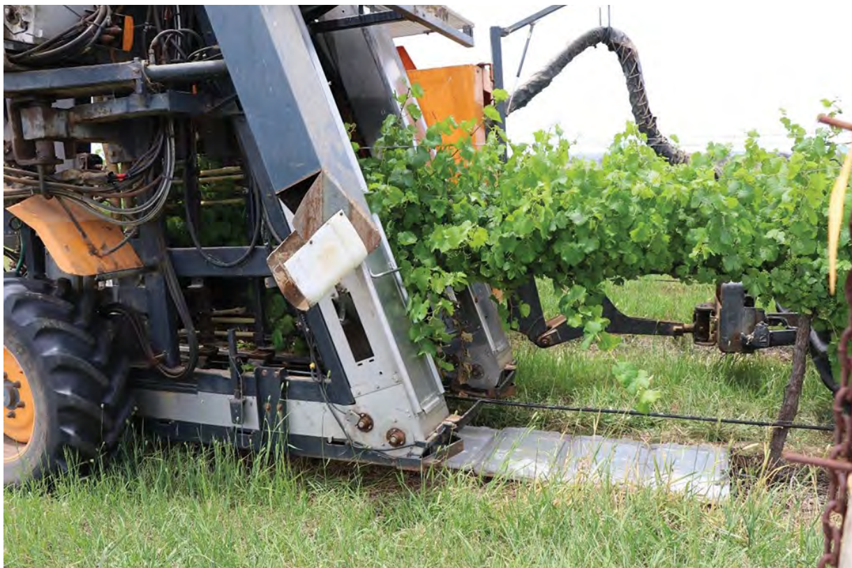
Figure 21. The harvester passes over white trays under the vine to gauge how much debris is removed by the shaker.
