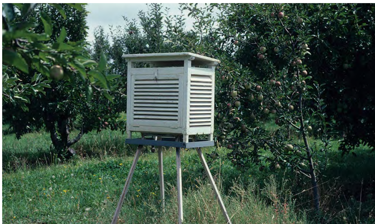
Figure 137. A Stevenson screen is the recommended housing for temperature recording in the orchard.
