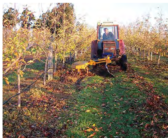
Figure 160. The Sadie sweeper moves leaf and pruning residue to the centre of the row for mulching. Photo: Crendon Machinery.
