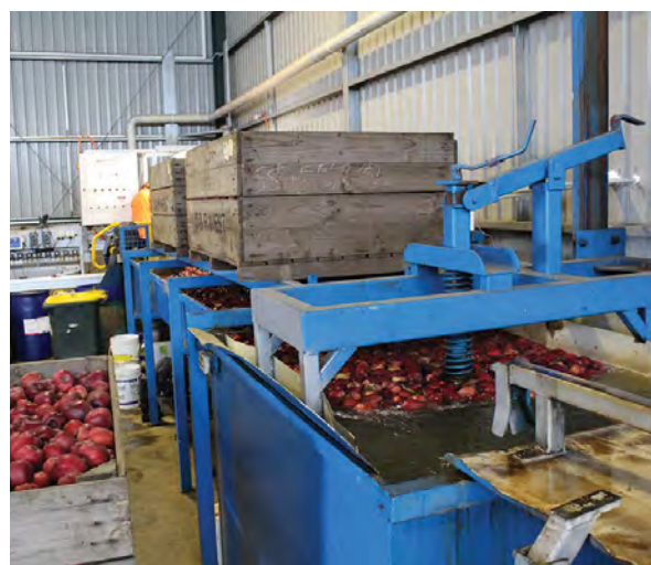
Figure 199. Dipping or drenching fruit in a fungicide solution as it comes into the packing shed.
